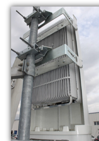
Nokia radio into the Hybrid Kit
